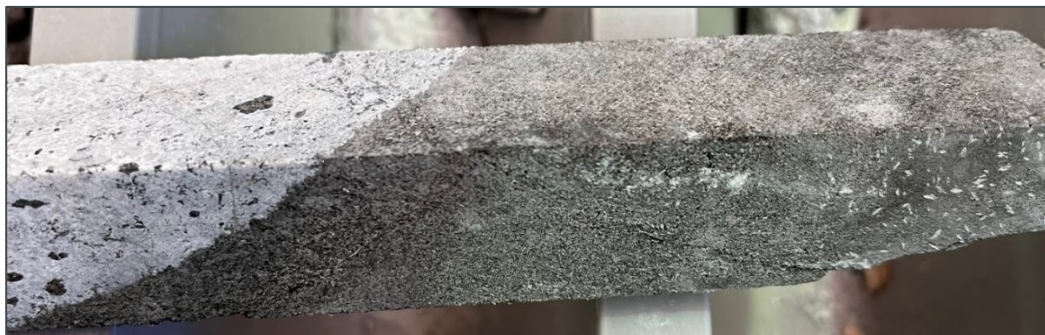
Figure 10: AHID0024: Section of core from 0.85m @ 0.34\% \text{Li}_2\text{O} , 3,392ppm Cs, 4,222ppm Rb, 51ppm TI from 368.75m with the Li-Cs-Rb-Tl anomalism within the dark biotite-rich interval on contact with the plagioclase-biotite porphyry.
